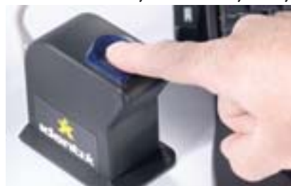
Put a finger on it and the reader checks your fingerprint against a database of fingerprints.
